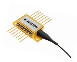
The 785nm series laser diodes are fabricated in a hermetically sealed 14-pin butterfly package. The laser diodes contain a monitor photodiode, thermoelectric cooler (TEC), and a thermistor to secure high-quality laser performance. Our laser products are Telcordia GR-468 qualified and in compliance with RoHS Directives.
